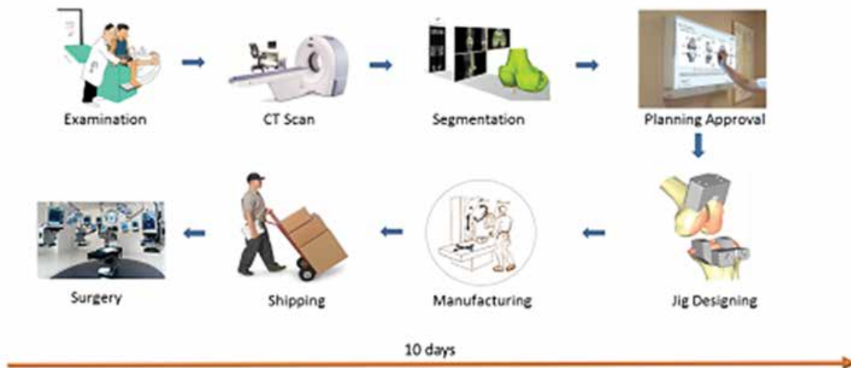
Fig 1. Pre-plan process flow for customized patient-specific implants
